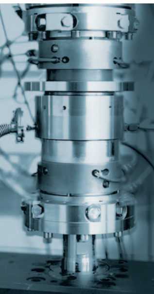
Helium leakage rate measurement
